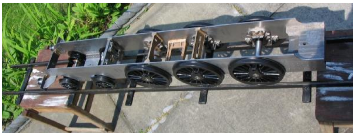
Partial frame assembly (Note the horizontal stretcher.)
